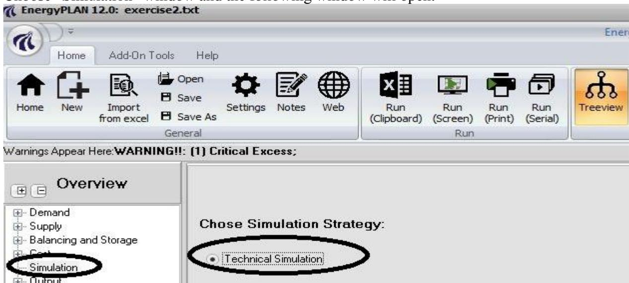
Make sure that the Technical Simulation is on. Change the Technical Simulation Strategy to ‘1 Balancing heat demands’
