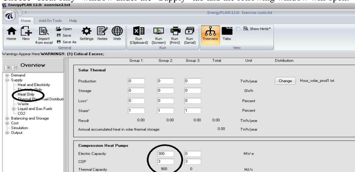
Place the cursor in the input squares and type in input values for the heat pumps.
